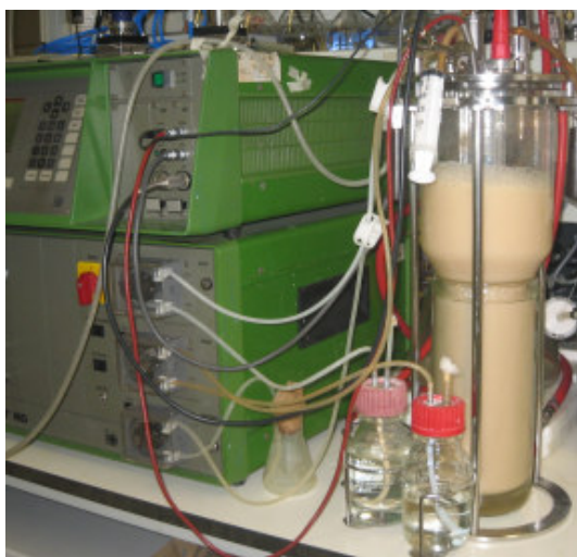
Fig. 4: High cell density cultivation of Cupriavidus necator in the ALR
