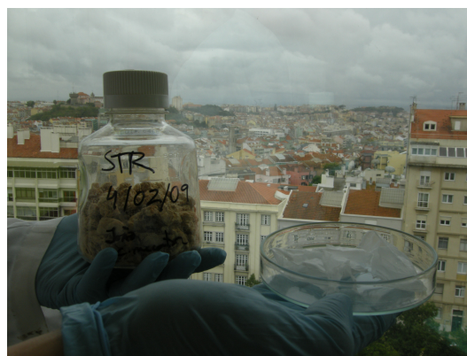
Fig. 2: Lyophilized cells and a film of bacterial P(3HB) obtained from waste glycerol.
